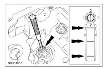
2. Measure the ball gauge with a micrometer.
